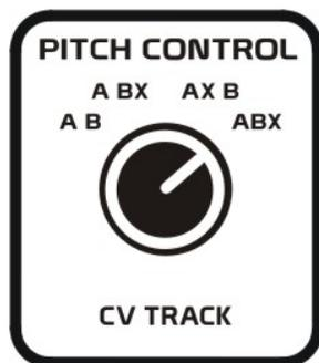
In the **A B** position, both oscillators will be controlled by MIDI notes received. In the **A BX** position, Oscillator A will respond to MIDI notes received, while Oscillator B will be controlled by an external voltage inserted into the CV IN jack.
