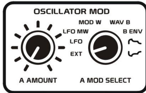
The MOD W setting will route the Mod Wheel messages from a MIDI keyboard to modulate Oscillator A's frequency. With your mod wheel set to 0, there will be no affect on Oscillator A's pitch. Increasing the value of your mod wheel will cause Oscillator A's frequency to increase accordingly.
